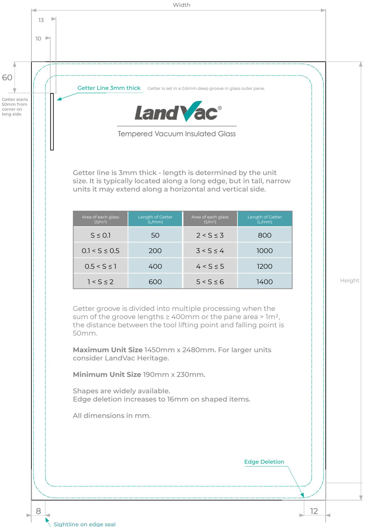
**Getter Line 3mm thick** Getter is set in a 0.6mm deep groove in glass outer pane.
